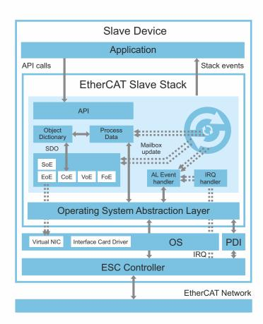
An EtherCAT Slave stack package may include a set of ready solutions for specific platforms and operating systems, such as:
