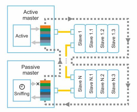
This feature is extremely useful for fault tolerance: any device connected to the bus is fully aware of slave's activity and can transparently acquire, or sniff, the data, which is transferred between master and slaves. There is no need to modify any slave devices, to add any additional signals, or to change the transfer protocol.
