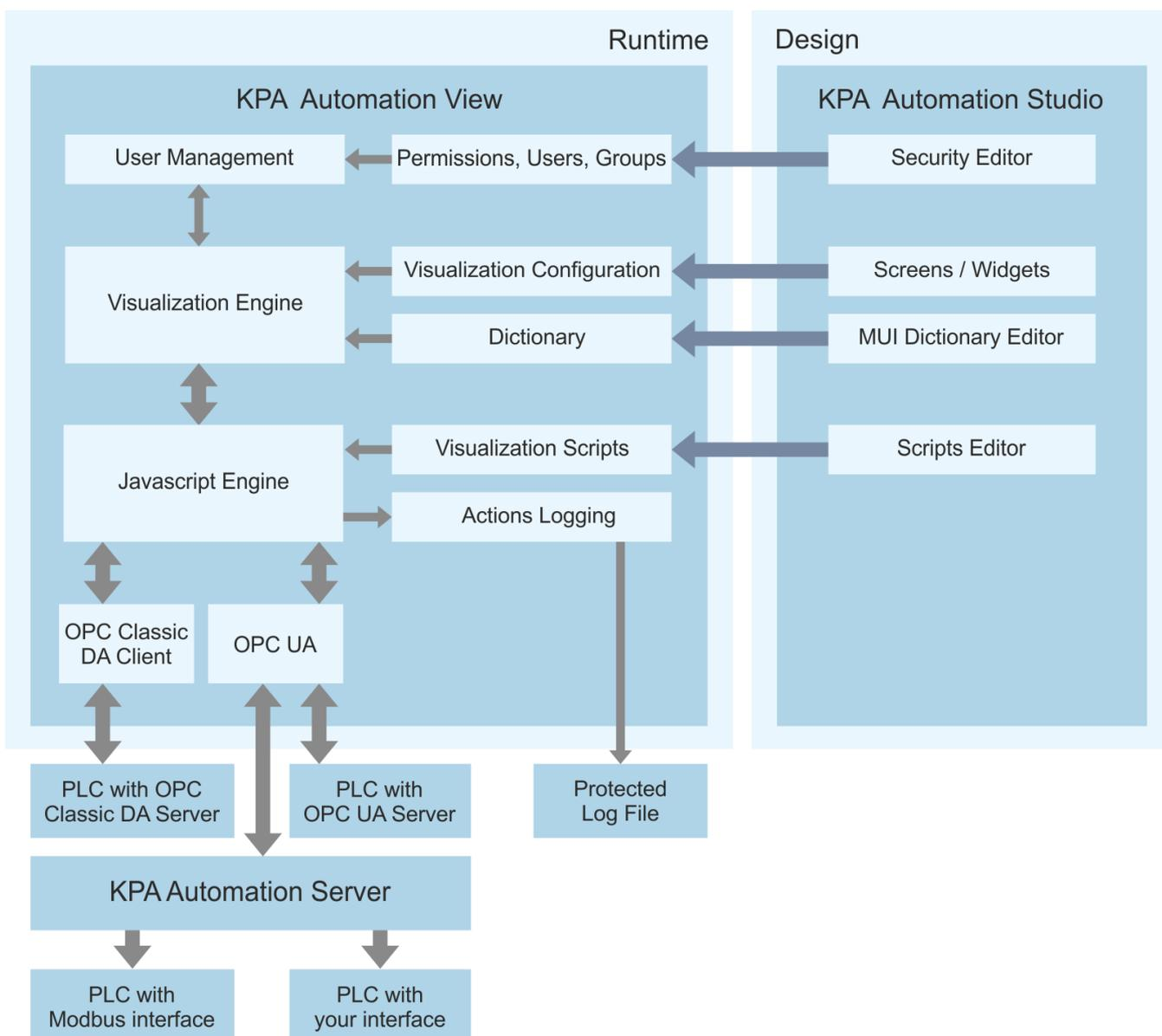
The delivered package of KPA Automation View includes **KPA Automation Studio** – integrated development environment with user-friendly drag-and-drop user interface for programming appearance and behavior of HMI controls.
