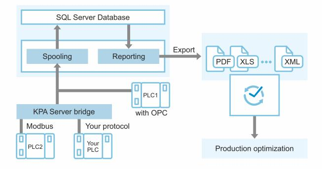
KPA Automation View in the package is used to select tags to be collected, to configure reports and to view ready reports. There is no need to keep KPAAutomation View running for data collection. All data is gathered by spooling service.
