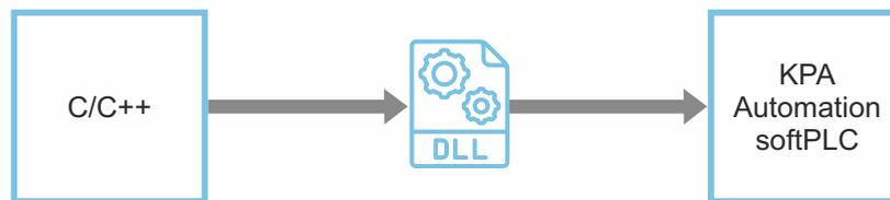
SDK includes Library Manager, which provides a function block source code template in the C/C++ programming language, and a sample with a custom function block.
