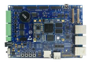
There are an Ethernet controller and PRUSS module on the board. Therefore, when using this board, data transfer is possible both through the internal interface and through the PRUSS module with support of hardware acceleration.
